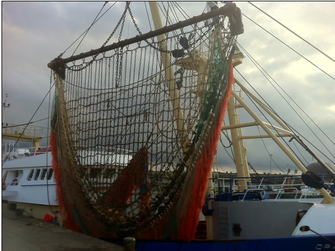
Plate 14.2 Traditional beam trawl with tickler chains and chain mat (Source: BMM, 2012)
